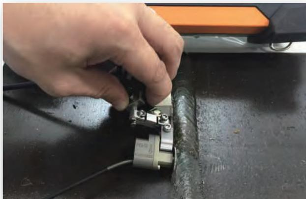
Butt Weld Inspection
